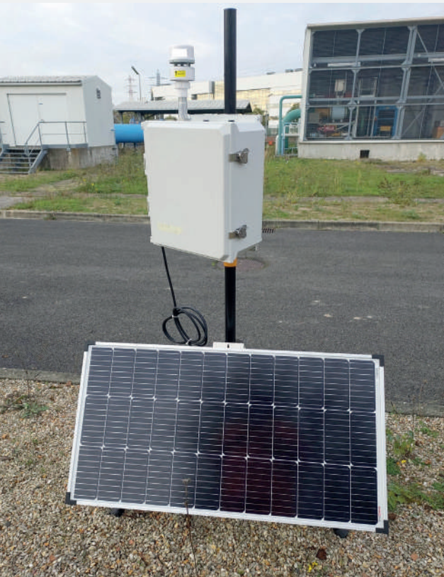
Controlled on-site testing of continuous methane monitoring solutions at our Alfortville site.
