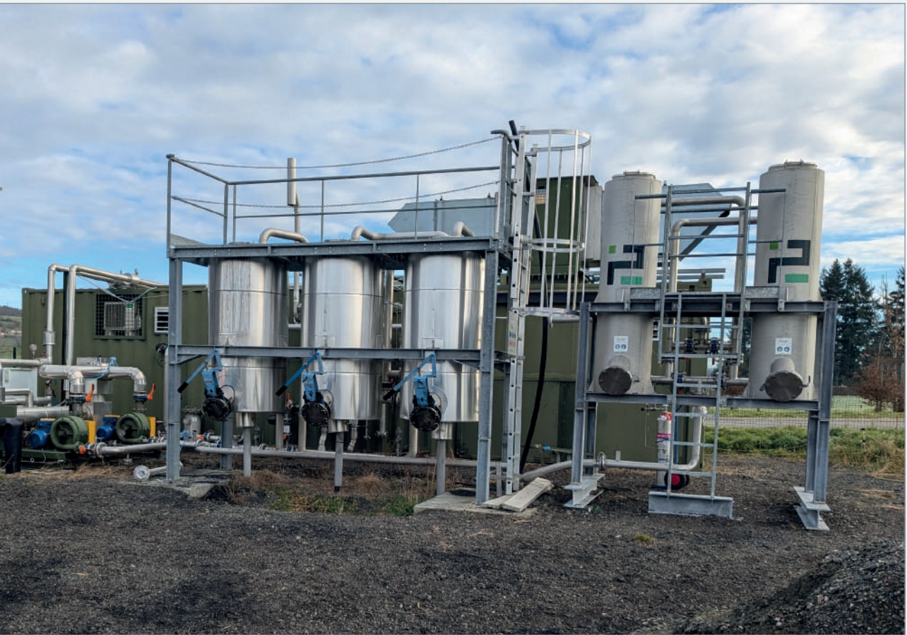
Desulphurisation and deoxygenation experiments using ferric salts at the Méthamoly biomethane site.
