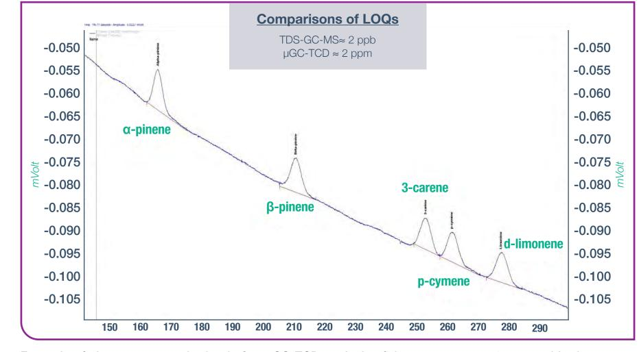
Example of chromatogram obtained after µGC-TCD analysis of the 5 terpenes at 2 ppmmol in the methane, CP Sil 5 CB column, (standard mixture prepared by NPL).
