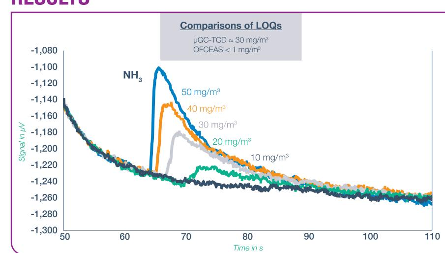
Chromatograms obtained after injection and analysis in  $\mu$ GC-TCD (PPU module) of NH $_3$  in the methane at 10/20/30/40&101 mg/m $^3$ .
