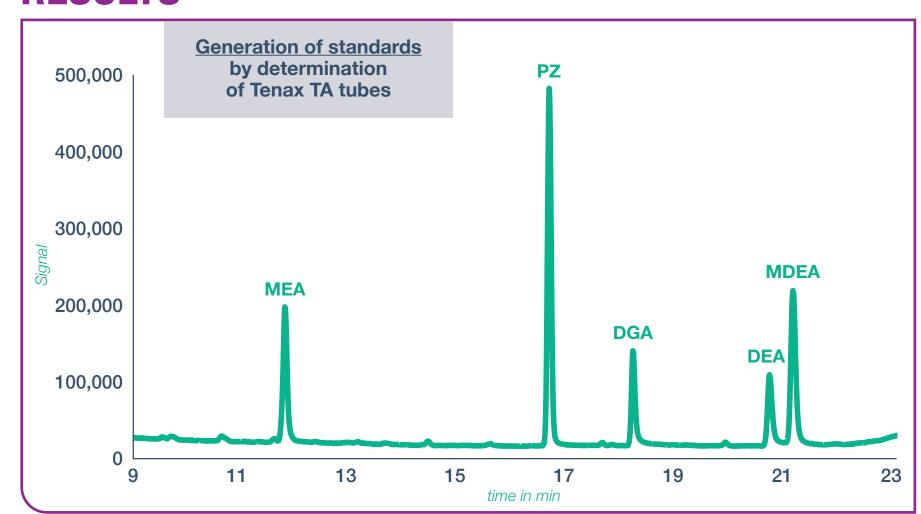
Example of chromatogram obtained after directly injecting 1  $\mu$ L of a 100 mg/L solution into the methanol of the 5 amines via an Rtx-Volatile Amine column.
